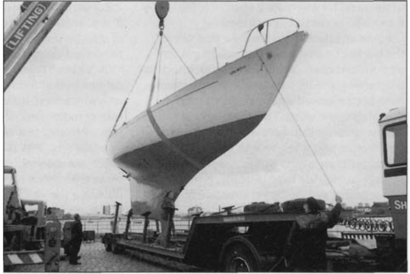
Fig. 2.4 Sailing Yacht 'Gipsy Moth IV'. In the construction of ships and yachts timber has been used to produce a wide variety of complex shapes. The material itself places little restriction on form but the production of geometries like that illustrated is highly labour intensive and therefore expensive. [Photo: The Maritime Trust]
