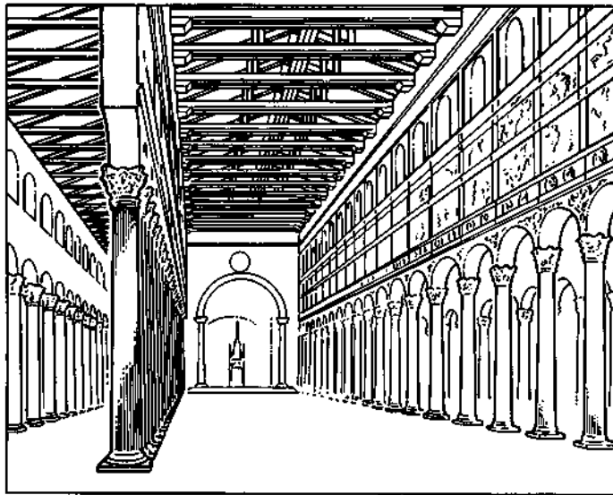
Fig. 6.8 Left. St Paul's Outside the Walls, Rome, 4th century CE. This perspective drawing illustrates well the advantage of using a triangulated timber roof structure rather than a vault. The thinness of the walls is well shown (after Piranesi).
