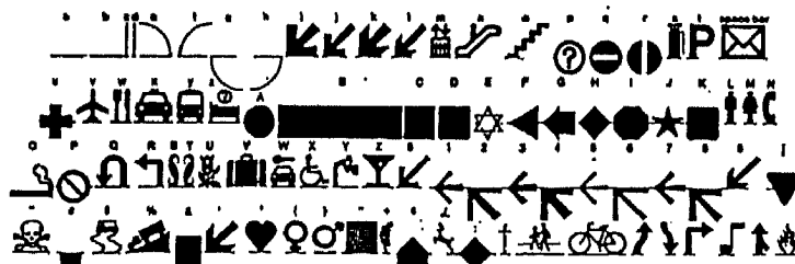
Fig. 14 General type styles with maximum readability. 1/2" cap height is legible up to 25', 3/4"-1" cap height is legible up to 50', 1-2" cap height is legible up to 100'.
